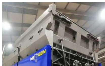
Hydraulic Raise / Lower Hopper Extensions
