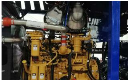
Tier 4 Final / Stage 5 - CATERPILLAR C9.3B 310Kw (420HP)
