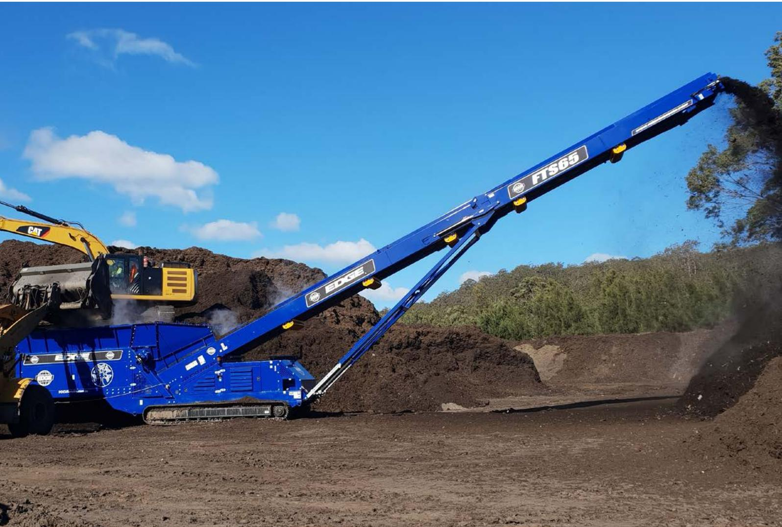
The EDGE FTS Mulch Master is a portable feed stockpiler that is specifically designed for the stockpiling of lower density, bulky materials such as mulch, compost and soils. The EDGE FTS Mulch Master combines traditional flipping and rotation with constant material flow to provide blockage free stockpiling whilst also preventing compaction, contamination and risk of combustion. It can accept material directly fed from wheel loaders, wood grinders, shredders, screeners or trommel screens.
