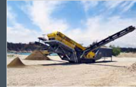
RM MSC5700M screening bank gravel
