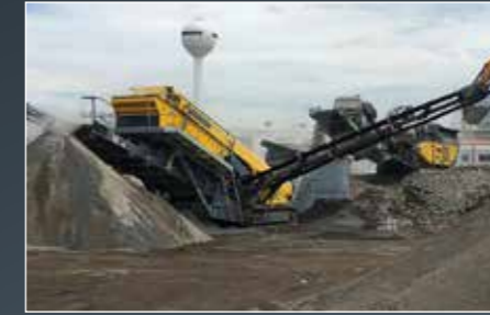
RM MSC6500M splitting up crushed material in 3 finished products
